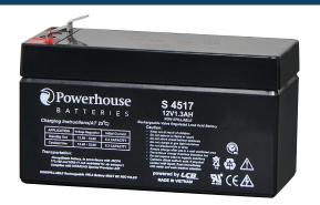
This 12V 1.3Ah sealed lead acid (SLA) battery is a compact battery for powering 12V equipment. It is commonly used in battery back up systems, alarm and communications systems and UPS units. Fitted with 4.8mm spade connection tabs, these batteries are easily user replaced in most equipment they are used in. Cells are fully sealed to prevent any leakage of electrolyte..
