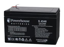
This 12V 12Ah sealed lead acid (SLA) battery is a compact battery for powering 12V equipment. It is commonly used in battery back up systems, alarm and communications systems and UPS units. Fitted with 6.3mm/F2 tab terminals, these batteries are easily user replaced in most equipment they are used in. Cells are fully sealed to prevent any leakage of electrolyte.
