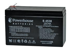
This 12V 7Ah sealed lead acid (SLA) battery is a compact battery for powering 12V equipment. It is commonly used in battery back up systems, alarm and communications systems and UPS units. Fitted with 4.8mm/F1 tab terminals, these batteries are easily user replaced in most equipment they are used in. Cells are fully sealed to prevent any leakage of electrolyte.
