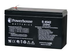
This 12V 9Ah sealed lead acid (SLA) battery is one of the most common size SLA batteries in use. It is commonly used in NBN boxes, battery back up systems, alarm and communications systems and UPS units. Fitted with 4.8mm spade connection tabs, these batteries are easily user replaced in most equipment they are used in. Cells are fully sealed to prevent any leakage of electrolyte.
