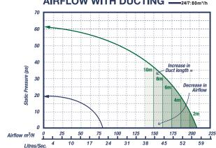
\*Airflow and pressure data tested as per international standard ISO 5801
