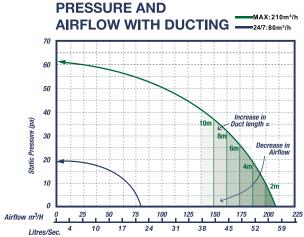
\*Airflow and pressure data tested as per international standard ISO 5801
