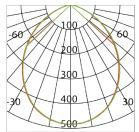
Unit: cd - C0/180,94.4 - C90/270,94.7 Photometric diagram shown is for 4000 K output.
