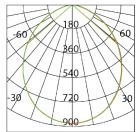
Unit: cd – C0/180,97.9 – C90/270,97.5 Photometric diagram shown is for 4000 K output.
