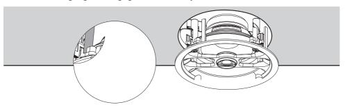
5. Place the grill on speaker. The grille will magnetically attaches to the rim of the
