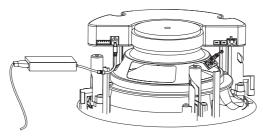
3. Insert the speaker into the hole and adjust the dog leg with the installation tool as shown.
