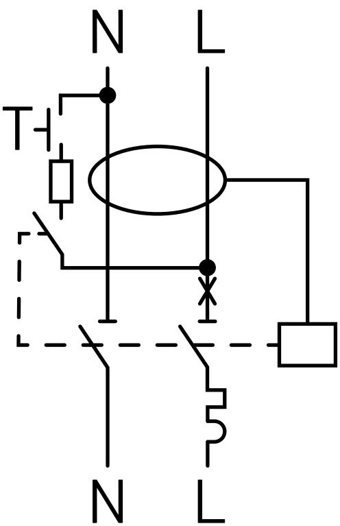
NHP MOD6+ RCBO 6kA 1 Pole and Switched N 32A C Curve 30mA Type A (2 screw)
