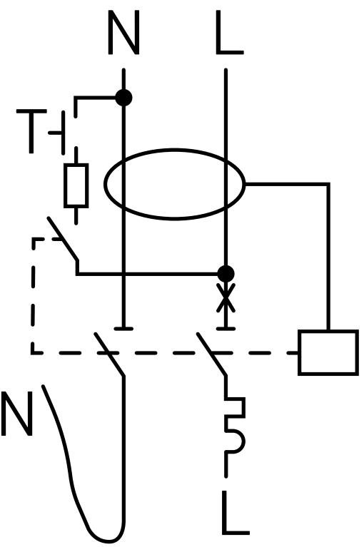
NHP MOD6+ RCBO 6kA 1 Pole and Switched N 32A C Curve 30mA Type A (Pigtail)
