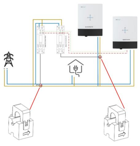
CT clamp arrow must face towards the property load and only clamp around 1 Live wire and not the neutral. CT clamp arrow must clamp around the Live cable of the PV string inverter facing towards the property load and only clamp around 1 Live wire and not the neutral.
