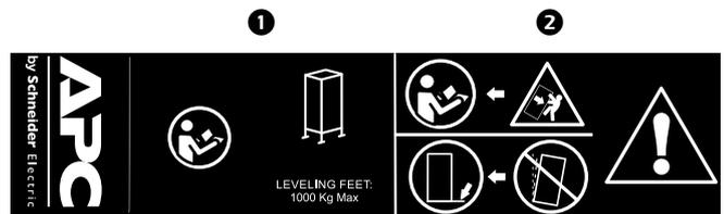
**Section 1:** Do not load additional equipment in to the cabinet before moving the cabinet on its casters. Once in place, lower the levelling feet. With the leveling feet lowered, the static cabinet can be loaded with up to 1,000 kg (2204.62 lb) of additional equipment.
