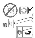
2. Place the cage nut tool on the other side of the cage nut and pull to snap it into position.
