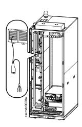
The UPS/Cooling connection wires are pre-installed to the Device COMM ports of the Interface Card Box and routed through the cable channel to the rear of the Micro Data Center. The connections are labeled **UPS-1** and **IDU-1**.
