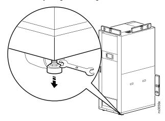
3. Using a level, adjust each foot until the cabinet is level and plumb.
