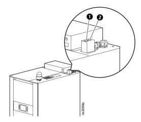
Alternatively, you can remove the top installation pipes and install the bottom cooling pipes (if included) instead. Install the bottom cooling pipes as shown so that the external connections to the suction line (1) and the liquid line (2) exit the bottom of the cabinet. See for instructions to remove the bottom plate.
