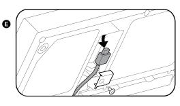
7. Route the NetBotz Handle wire through the display plate **G**. You can use the support brackets on the door rods for additional cable management **G**.
