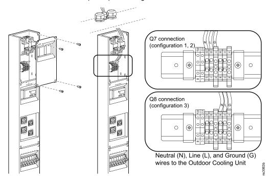
**NOTE:** Both Cooling Units must be controlled by the same breaker.
