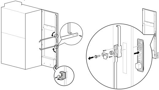
2. Install the NetBotz Handle kit and gear box (NBHN4340).
