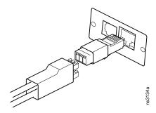
SRT6KRMXLI: Install the UPS-1 wire to Modbus port on the SmartSlot card. Ensure the pin with the black wire is inserted in to the chassy ground connection point (4).
