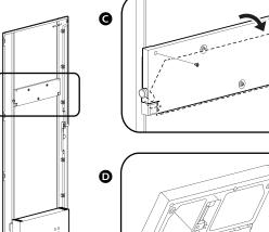
5. Remove the three Phillips head screws securing the display to the plate **①**.
