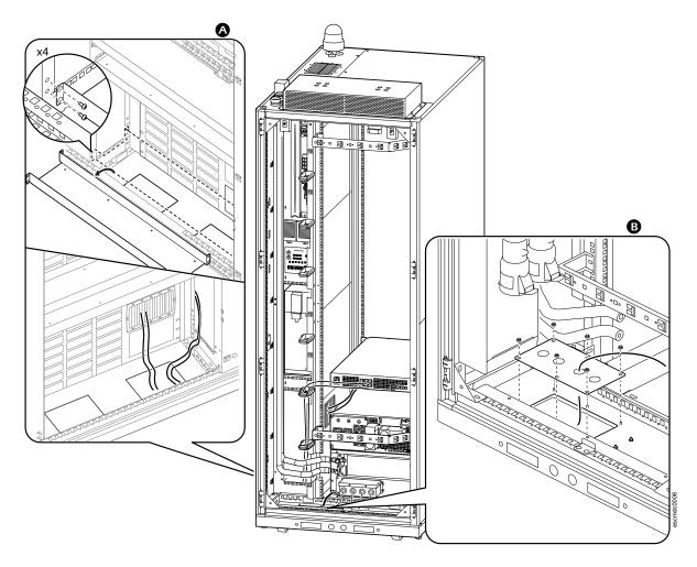
\*If needed, you can rotate the blanking panel 180° to place the optionally installed brush strips near the front of the Micro Data Center. The interior blanking panels are held in place with self-tapping Phillips-head screws.
