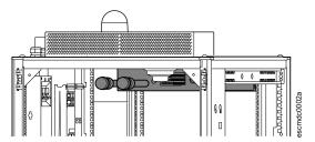
2. Install the two smoke sensors (included in ARFS600) to the mounting bracket near the top of the Micro Data Center. Use the screws and wing nuts included with the smoke sensors. If needed, you can move the mounting bracket down a few spaces on the mounting rails for easier access. Connect the smoke alarms to the fire suppression unit as directed in the wiring diagram for accessories included with the smoke sensors.
