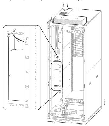
**NOTE:** For SRT192RMBP, you must ground the battery pack to the rear cabinet frame. Connect the provided grounding wire and pan-head screws to the battery pack as instructed in the battery pack installation manual. Use the pre-installed M4 screw and serrated washer to make the connection to the Micro Data Center Frame.
