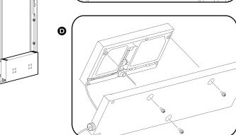
6. Remove the cable bracket and retain the bracket screw. Remove the micro-HDMI cable from the display and set the display aside **9**.
