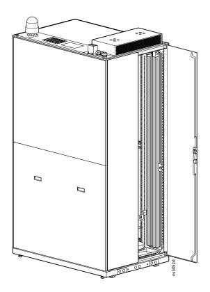
Follow the Rack PDU installation instructions to Install the Rack PDU units in the 0 U mounting spaces at the rear of the cabinet. Connect the Rack PDUs to the designated IEC 309 sockets on the power panel. If you only have one Rack PDU, connect it to the Rack PDU A power socket. If an ATS is not included in this configuration, connect the NetBotz Rack Monitor 250 into Rack PDU A. See Power Panel Description, page 31for details.
