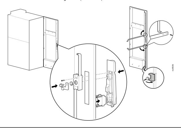
3. Attach the included cable assembly to lock connector port ( a) and the proximity reader cable ( b).
