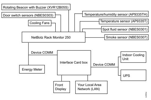
**NOTE:** Rack PDUs, ATS units, KVMs, and fire suppression units cannot be monitored through the front display or the Web UI of the EcoStruxure Micro Data Center. Metered/Switched Rack PDUs, ATS units, and KVMs can be monitored through their own user interfaces (see the documentation for each device). If compatible, the fire suppression unit may be connected to your building fire panel.
