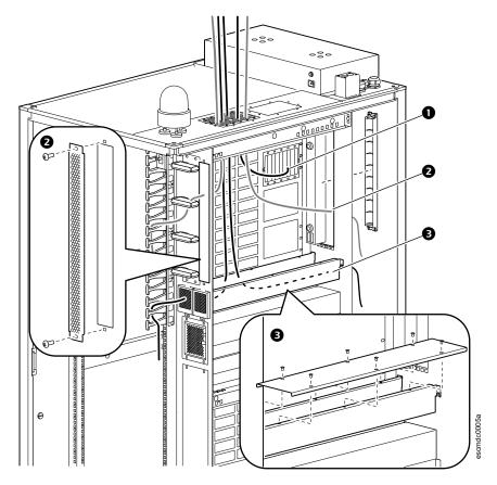
There is an additional compartment for cable storage at the top of the EcoStruxure Micro Data Center. Cables can be routed to and from the compartment from the interior, rear side of the EcoStruxure Micro Data Center, then accessed from the top.
