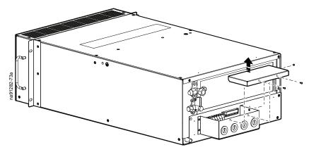
2. Connect the RS485 converter cable to the leftmost RS485 ports on the Indoor Cooling Unit **3**.
