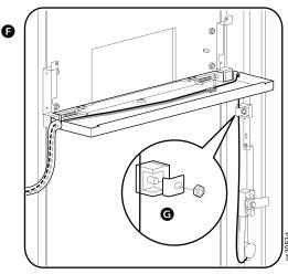
8. Route the NetBotz handle wire through the brush strips and cable bridge to the rear of the rack (1). Connect the wire to a Handle port\* on the NetBotz 250. If needed, use the RJ45 coupler (included with the handle kit) to connect the handle wire to a Cat 5 patch cable. You can wrap excess cable length around the front display.
