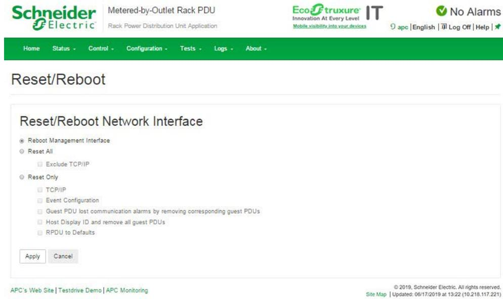
**Reset All:** Clear the **Exclude TCP/IP** checkbox to reset all configuration values; mark the **Exclude TCP/IP** checkbox to reset all values except TCP/IP and EAPoL.
