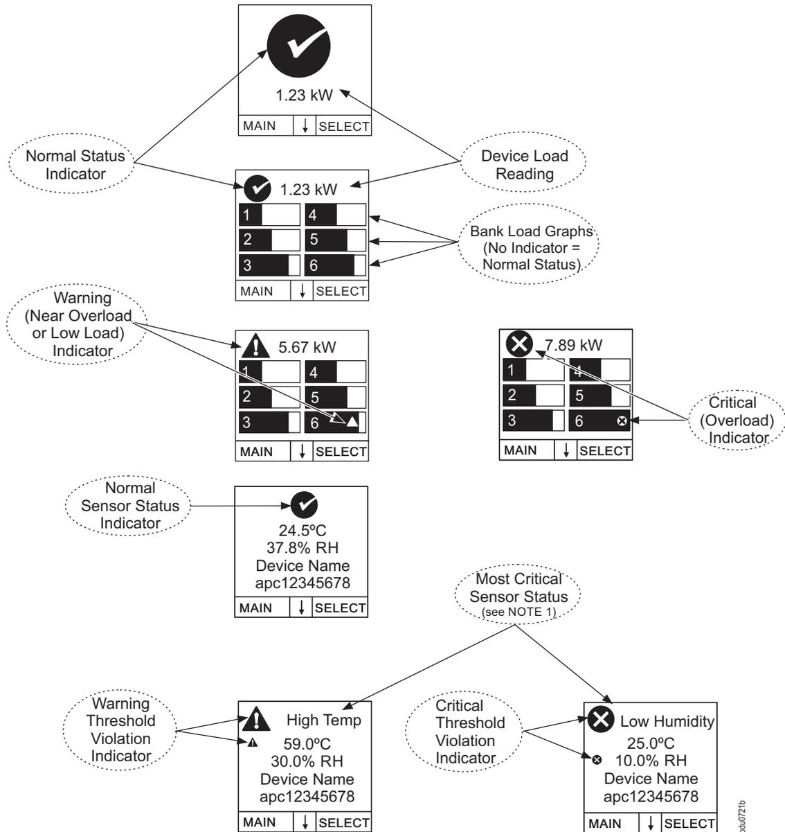
**NOTE 1:** The simplified LCD screens will show device load alarms only when no banks are present OR bank load alarms only when banks are present. Phase and Outlet alarms and warnings will NOT be displayed.
