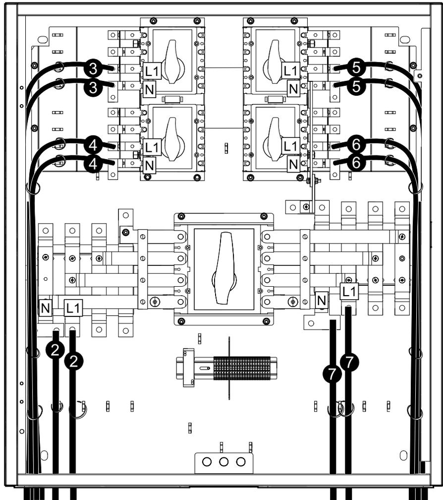
3. Connect the UPS input cables/UPS bypass cables from UPS 1.
