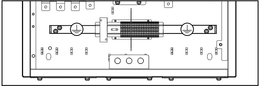
2. Connect the input cables from utility/mains.
