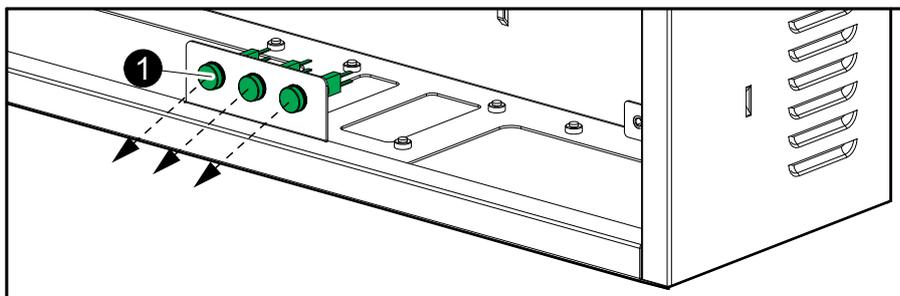
2. Install three round blanking plugs (not provided) in the holes in the inner door.
