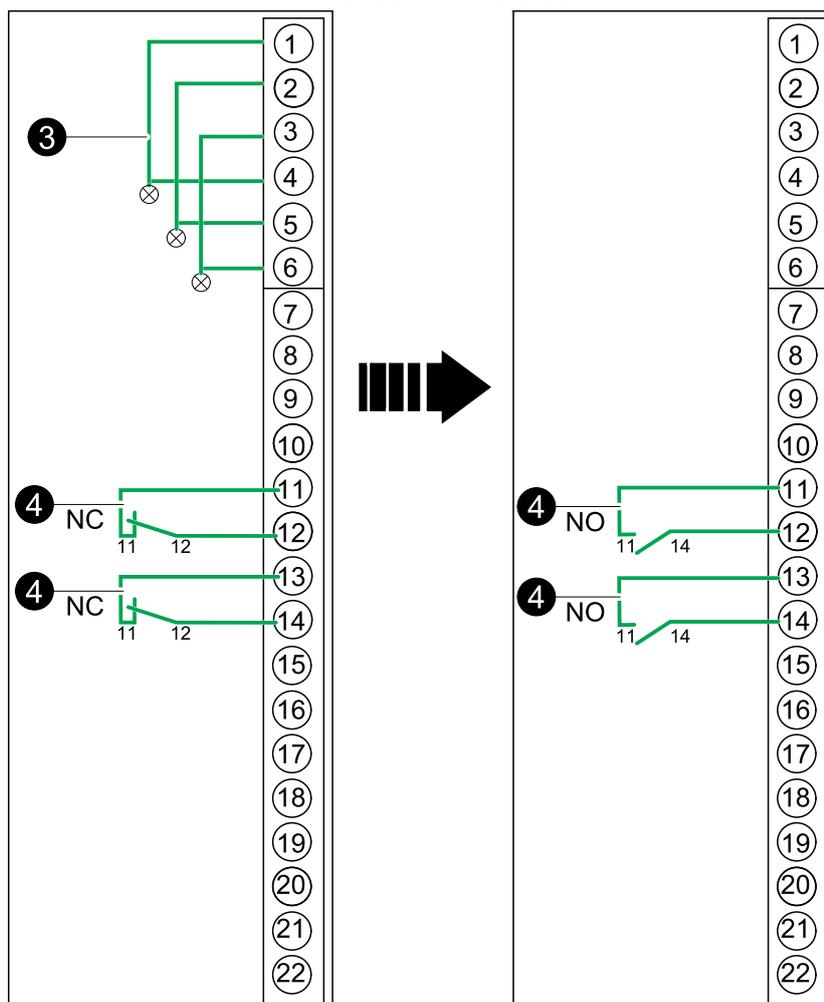
4. On the control terminal block, modify the internal connection for the MBB AUX switches (pin 11-14) from Normally Closed (NC) to Normally Open (NO).
