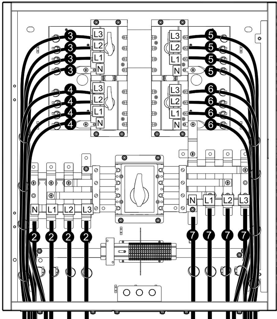
3. Connect the UPS input cables/UPS bypass cables from UPS 1.
