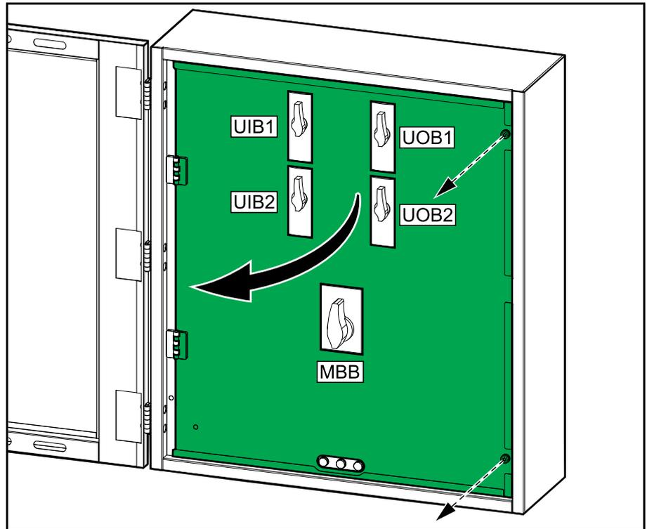
4. Mount the parallel maintenance bypass panel to the wall.
