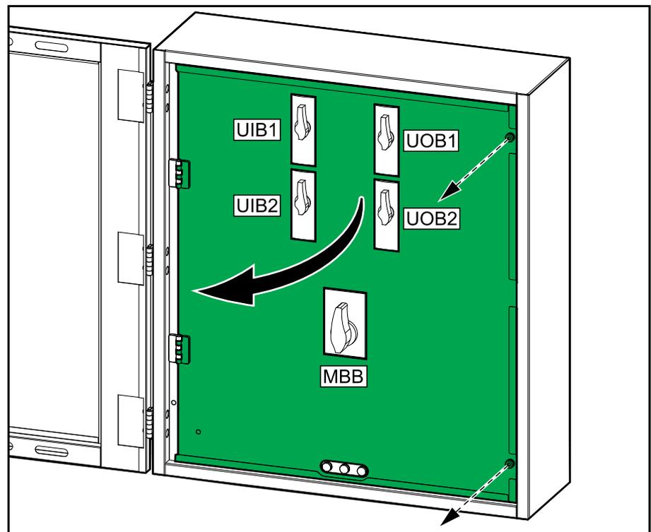
8. Measure for and verify ABSENCE of voltage on each input/bypass busbar, UPS input/UPS bypass busbar, UPS output busbar, and load busbar before continuing.
