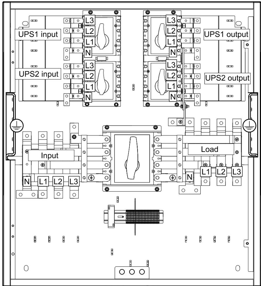
9. Disconnect and remove all power cables from the parallel maintenance bypass panel. See Connect the Power Cables on GVSBP10K30H, page 32, Connect the Power Cables on GVSBP40K50H for a 3:1 UPS System, page 33, Connect the Power Cables on GVSBP40K50H for a 3:3 UPS System, page 36, Connect the Power Cables on GVSBP60K120H for a 3:1 UPS System, page 37, or Connect the Power Cables on GVSBP60K120H for a 3:3 UPS System, page 40 for details.
