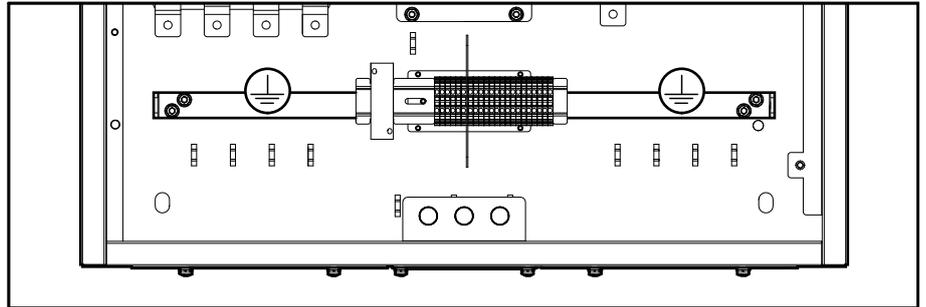
2. Connect the input cables/bypass cables from utility/mains.
