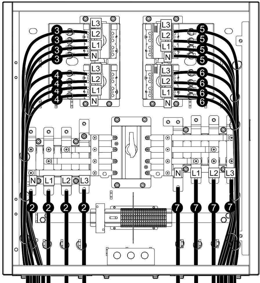
3. Connect the UPS input cables from UPS 1.
