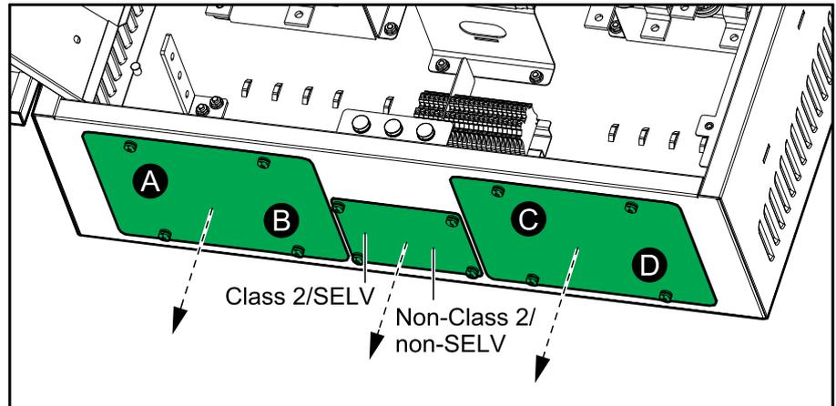
2. Drill or punch holes for power cables and signal cables or grommets in the gland plates. UPS input (A), input (B), load (C), UPS output (D).
