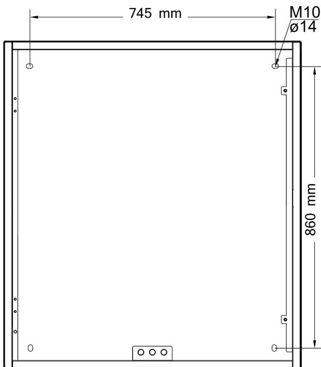
2. Drill holes in each of the four marked locations and mount the anchor bolts.
