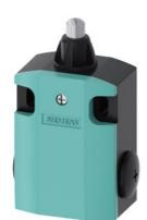
Position switch Metal enclosure 56 mm wide Device connection 3 x (M20 x 1.5) 1 NO/1 NC quick action contacts Rounded plunger, with 3 mm overtravel made of stainless steel Actuating/restoring force 30 N only available as complete unit
