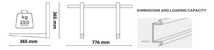
Cross Bar equipped with built in spirit level with very easy installation. Hot galvanized to ensure longevity & service life. OEM packaging.
