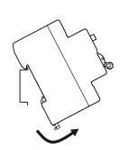
WARNING: If RCD trips it maybe caused by either, overload, short circuit or earth leakage. The installation should be checked before resetting RCD.
