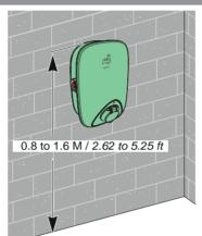
■ Check the installation area before marking it on the wall. It is recommended to situate the top of the charging station between 0.8 to 1.6 m / 2.62 to 5.25 ft above the ground.
