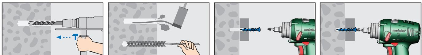
Plasterboard - No pre-drilling required (Warning: Over-drilling will decrease load capacity.)
