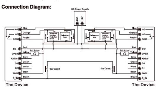
Remarks: The Door Contact must be installed and connected as the diagram. Let's name the two Devices as "A "and "B" for two doors "1" and "2"
