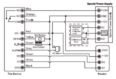
Attention: Install a 1N4004 or equivalent diode is needed when use a common power supply, or the reader might be damaged. (1N4004 is included in the packing)
