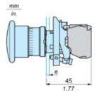
e : clamping thickness: 1 to 6 mm / 0.04 to 0.24 in.
