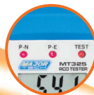
Correct Wiring Indication
