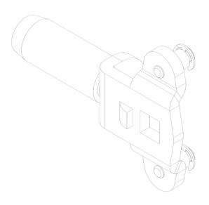
CONCEPT Door Handle, Locking Roller Cam, Three Point, suits  $\ensuremath{\mathsf{CPL}}$  and  $\ensuremath{\mathsf{CPR}}$
