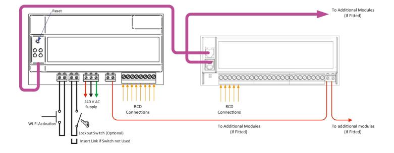
Connection / Wiring Diagram
