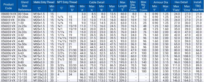
All dimensions except NPT are in mm. Intermediate thread sizes are available on request. NPT threads should be tightened 'wrench tight'.
