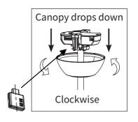
Replace Canopy by sliding upward and re-fixing by twisting Anti clockwise.
