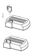
2. Finalise Installing your Skyfan DC ceiling fan (must be installed by licensed and qualified tradesperson. Note: If fan has already been installed, turn off main power supply, remove fan upper canopy by twisting in a clockwise direction and lowering to expose receiver box. Then insert App control module. This can be completed without removing the receiver but should be completed by a licensed and qualified tradesperson.
