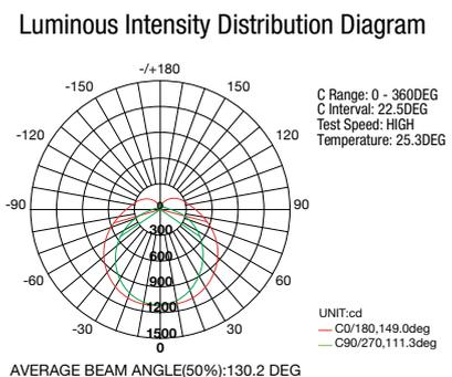
Product No: TLDB34640S AAI Figure at 4000k CCT    Product No: TLDB34640S Luminous Intensity Measure at 4000k CCT
