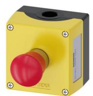
Enclosure for command devices, 22 mm, round, Enclosure material metal, Enclosure top part yellow, 1 control point metal, A=EMERGENCY STOP mushroom pushbutton red, 40 mm, rotate-to-unlatch, Control point in center, 1 NC, screw terminal, floor mounting, 1xM20 each on top and bottom
