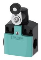
position switch plastic enclosure 50 mm, device connection 2 x (M20 x 1.5) 1 NO/1 NC quick action contacts, twist lever with plastic roller 19 mm
