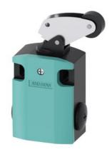
Position switch Metal enclosure 56 mm wide Device connection 3x (M20x 1.5) 1 NO/1 NC slow-action contacts Angular roller lever, metal lever and plastic roller 22 mm
