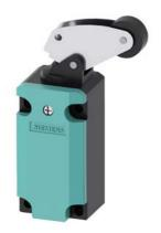
Position switch Metal enclosure 40 mm according to EN 50041 Device connection 1x (M20 x 1.5) 1 NO/1 NC slow-action contacts Angular roller lever and plastic roller 22 mm
