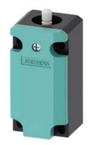
Basic switch for position switch 3SE513 Enclosure plastic according to EN 50041, 1 x (M20 x 1.5) 1 NO/1 NC slow-action contacts without actuator head
