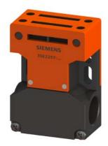
Safety position switch with separate actuator Molded-plastic-encapsulated short enclosure, 3x(M20x1.5) lateral and face-end operation slow-action contact 1 NC, Pull-out force 5 N Supplied without actuator
