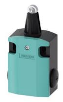
Position switch Metal enclosure 56 mm wide Device connection 3x (M20x 1.5) 1 NO/1 NC slow-action contacts Roller plunger with Stainless steel roller 13 mm
