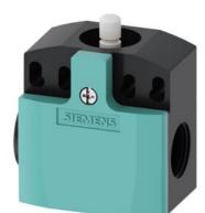
position switch plastic enclosure 50 mm, device connection 2 x (M20 x 1.5) 1 NO/1 NC slow-action contacts, rounded plunger
