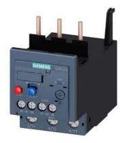
Overload relay 40... 50 A Thermal For motor protection Size S2, Class 10 Contactor mounting Main circuit: Screw Auxiliary circuit: Screw Manual-Automatic-Reset
