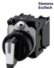
Selector switch, illuminable, 22 mm, round, plastic, white, selector switch, short, 3 switch positions I>O<II, momentary contact type, 10:30h/12h/13:30h, with holder, 1 NO, 1 NO, screw terminal
