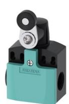
position switch plastic enclosure 50 mm, device connection 2 x (M20 x 1.5) 1 NO/1 NC slow-action contacts, twist lever with plastic roller 19 mm
