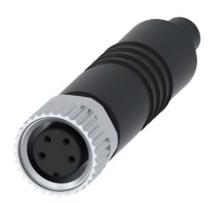
Coupling M8 with connection cable, 5 m long for M8 connector 4-pole, for 3SE66 magnetically-operated switch
