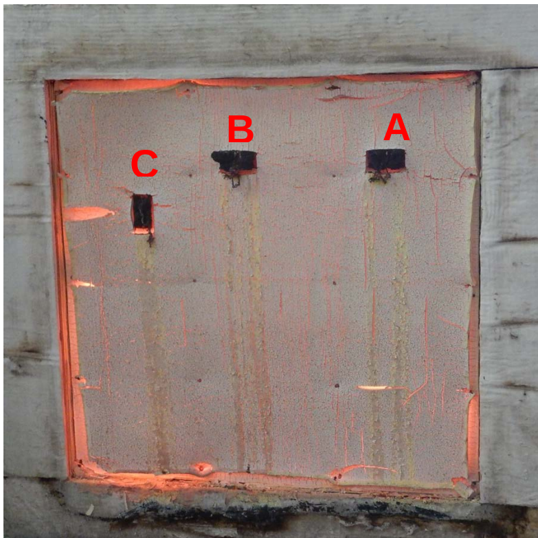
Figure A6.4. Exposed face of specimen after the end of the fire-resistance test.
