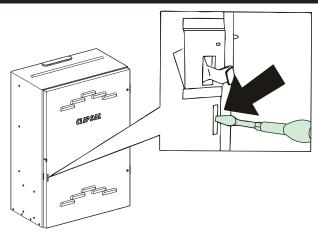
1. Break out knockout slot from the inside of door
