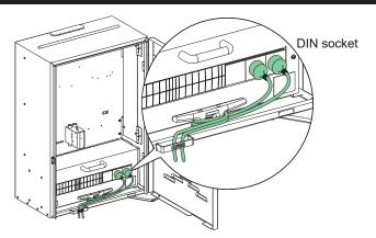
Pass the leads through cable protection slide at the bottom opening and tie off before plugging into socket outlet
