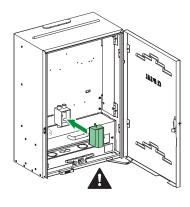
**5.** Reassemble the fuse carrier to base portion
