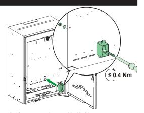
Use accessories provided in kit for fixing meter isolation link on meter panel
