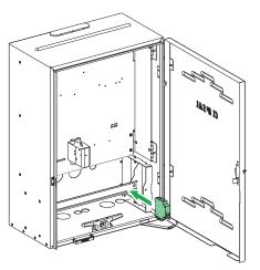
2. Add DIN mounted protection device as required Note: DIN is suitable for 21 module of 18 mm each
