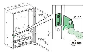
3. Reverse the locking strap in same position and reassemble it with the screws
