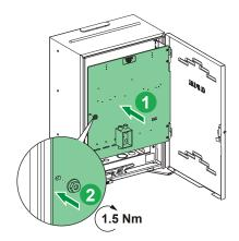
After wiring to meter isolation link from rear side of meter panel, push back meter panel to its original position
