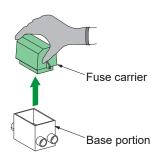
**2.** Pullout meter isolation link fuse carrier from base portion
