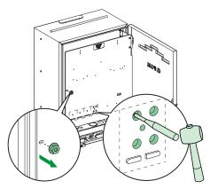
Knockout meter isolation link mounting and cable entry holes on meter panel as required
