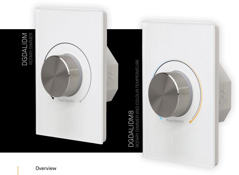
A Diginet DALI Wall Plate Dimmer with a built-in DALI bus power supply to power a DALI line and control up to 50 DALI drivers. Only a mains connection (Active and Neutral) and DALI connection (DA/DA) are required. No external DALI power supply or other equipment is required. Also no programming of the device or DALI drivers is required.
