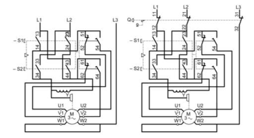
Control of Single-Speed Reversing Motor 3-Phase switching, Reversing by 2-Phase Inversion
