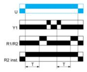
Function P: Pulse Delayed Relay with Fixed Pulse Length
