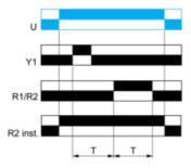
Function N: Retriggerable Interval Relay with Control Signal On
