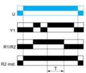
Function O: Retriggerable Interval Delayed Relay with Control Signal On
