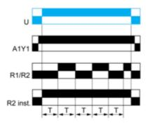
Before power-up Y1 should be permanently connected to A1. 2 timed outputs (R1/R2) or 1 timed output (R1) and 1 instantaneous output (R2 inst.)
