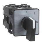
Cam changeover switch, Harmony K, multifixing, plastic, 2 poles, position 0, 45 degree, 20A, 45x45mm, metallic legend, marked 2/0/1, 35mm black handle
