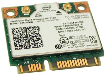
The HMIYMINWIFI2 is the IEEE 802.11ac/a/b/g/n 2 x 2 MIMO WLAN and Bluetooth.
