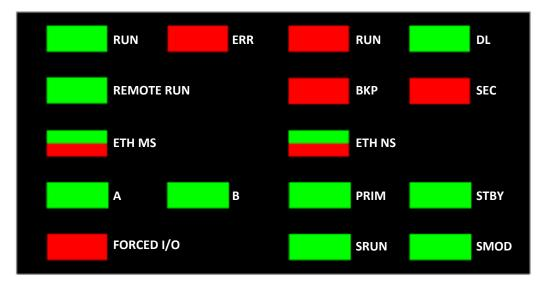
**NOTE:** The **SRUN** and **SMOD** LEDs apply only to safety controllers. The **SEC** LED is not used.
