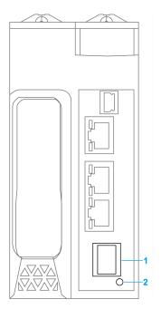
**1** SFP socket for copper or fiber-optic Hot Standby link connection
