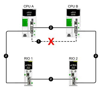
1 Hot Standby fiber optic link between controller A (CPU A) and controller B (CPU B)
