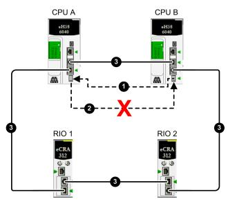
1 Operational Hot Standby fiber optic link from controller B (CPU B) to controller A (CPU A)
