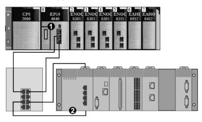
**1** M580 CPU: The CPU on the M580 local rack. In this example, you will enable this CPU's embedded scanner service as a local slave device (or target, **T**).
