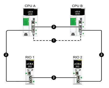
1 Hot Standby fiber optic link between controller A (CPU A) and controller B (CPU B)
